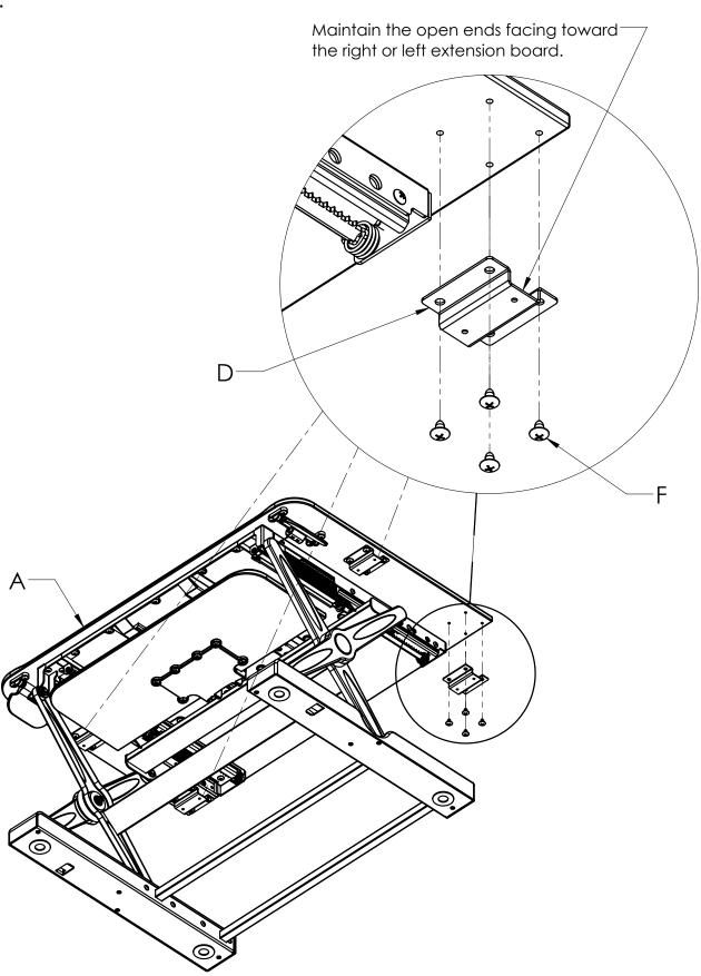
Step 2: First insert either of the extension board (B or C) into the brackets (D). Next, use 2 knobs (E) on each bracket when fastening this side. Do the same on the other side, and use the rest of 4 knobs to fasten this side.
